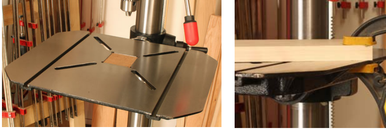
The generous cast iron table (left) has a replaceable center and X-shaped grooves that make securing work pieces easy. The flat edges of the table (right) make using common clamps to secure work pieces fast and secure.
