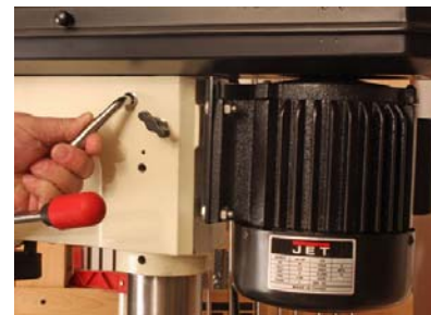
The powerful 3/4HP motor is mounted on an easy to use belt tensioning system. The locks and tensioning handle are easily accessible.
