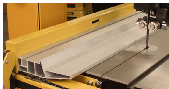
The large, extruded aluminum fence can be used lying flat on the table (left) or upright (right). It can also be moved front to back to best support the job at hand.
