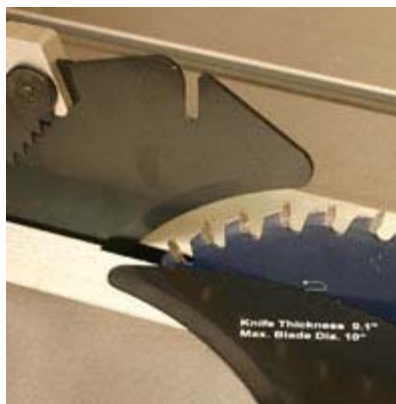
(Left) Standard and thin kerf splitters and low profile riving knives (Right) are available, all with beveled leading edges.
