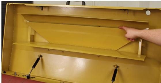
The top of the cabinet opens for easy access to the drums and shows the special dust system that helps keep this machine performing.
