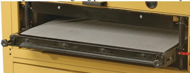
The conveyor belt runs on a precision cast iron table for flatness and consistency.
