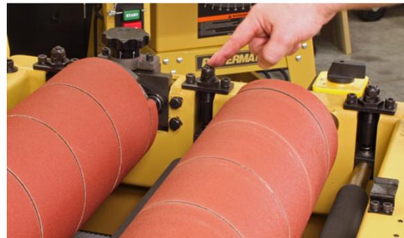
The pressure rollers are easily adjusted with these tough but simple mechanisms located up top for easy access.
