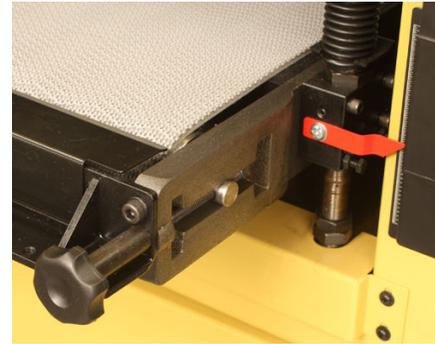
The conveyor is driven by a two-speed gearbox (left) that is shifted while the belt is running. Each side of the conveyor has an easy adjuster (right) for belt tracking and tension
