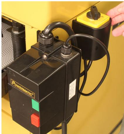
Industrial-tough controls, including a full magnetic switch protect the POWERMATIC Dual Drum Sanders.
