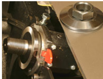
The 1"-diameter arbor (left) runs in large, high-quality ball bearings to insure long-lasting, smooth operation. We use a serpentine belt (right) to drive the arbor because of its smooth operation, low slippage and drastically reduced heat generation as compared to typical V-belt styles.
