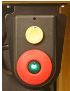
The magnetic switch protects the motor from harmful power fluctuations. It also prevents unexpected startups should the power go out and then come back on again.
