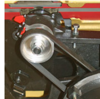
The 1"-diameter arbor (left) runs in large, high-quality ball bearings to insure long-lasting, smooth operation. We use a serpentine belt (right) to drive the arbor because of its smooth operation, low slippage and drastically reduced heat generation as compared to typical V-belt styles.
