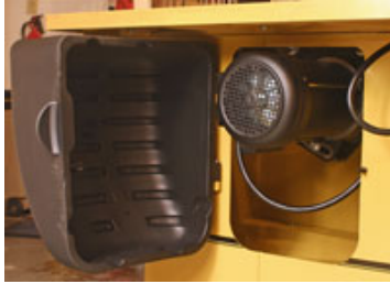
The large cabinet door enhances dust collection when closed but affords plenty of access to the cabinet interior when needed.
