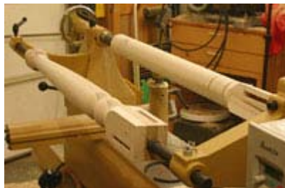
(Left) The Comparator mounts are standard and make turning sets of duplicate projects much easier. (Right) Being able to locate a sample directly behind the piece being turned makes it easy to match diameters and shapes to produce virtually identical turnings.
