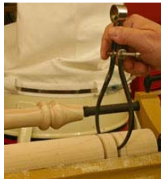
(Left) The Comparator mounts are standard and make turning sets of duplicate projects much easier. (Right) Being able to locate a sample directly behind the piece being turned makes it easy to match diameters and shapes to produce virtually identical turnings.
