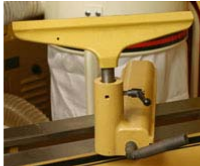
(Left) The 14” ductile iron tool rest is designed for safe, accurate use. (Right) Though bored for a 1”-diameter post, the special groove makes it possible to use smaller tool rests and still lock them securely.
