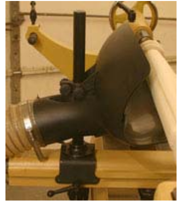
The Adjustable Dust Port accessory does a great job of removing fine sanding dust from the work area.
