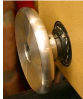
An adjustable bearing, located behind the hand wheel allows the user to tune out endplay should it develop in years to come, saving a trip to the service center and lots of potential downtime.
